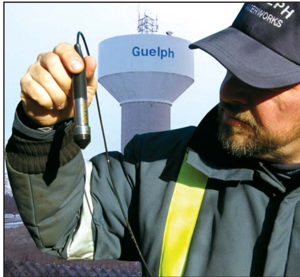
Groundwater monitoring using Diver dataloggers in the City of Guelph, Ontario, Canada
