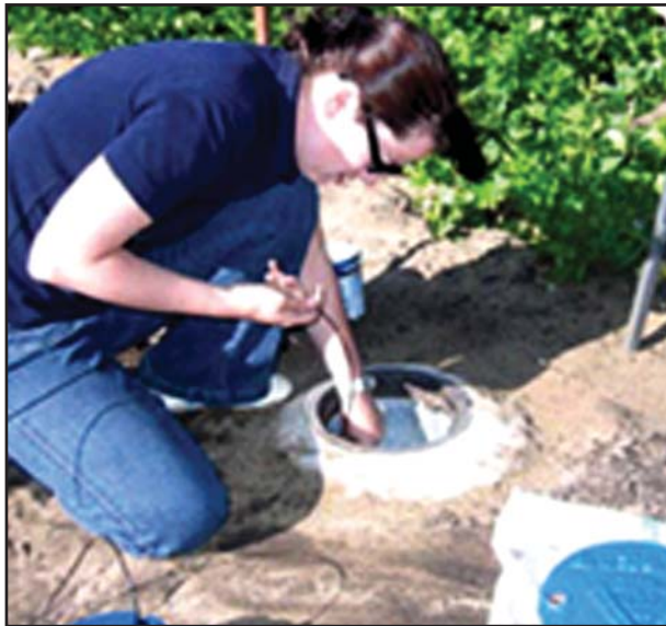
Suspending Divers into wells for continuous monitoring.
