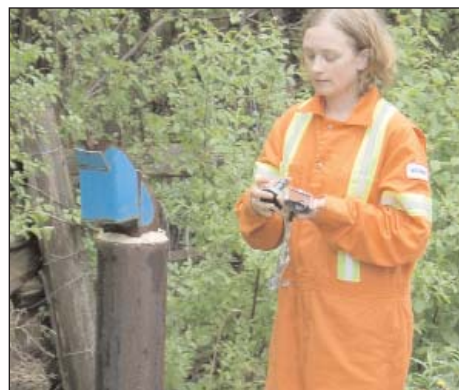
Programming Diver Dataloggers for continuous monitoring using hand-held PC
